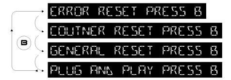
To switch between the different parameters, repeatedly press the B button. After selecting the parameter to be used, press the A button to activate one of the actions described below.
