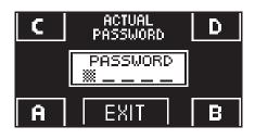
• Enter the default primary password "A-A-A-A-A" pressing 5 times the button A. (If the primary password is not the default password, since it had already been changed before, enter the currently-used primary password).
