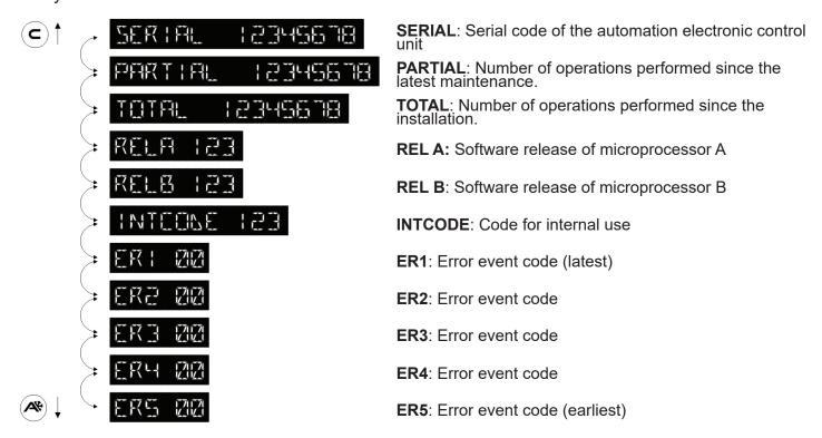
Scroll the sequence using the A (down) or C (up) buttons.
