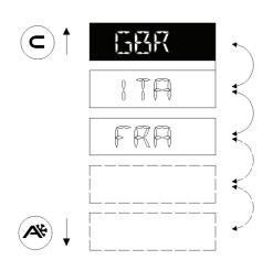
When installed for the first time, the selector shall automatically switch to the language selection menu.
