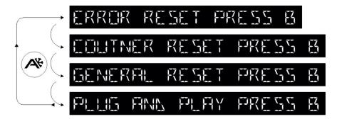
To switch between the different parameters, repeatedly press the A button.
