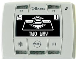
Each time, before using the R-DSEL digital selector, the user is prompted to enter the relevant password. If no operations are performed for about 6 seconds, the R-DSEL programmer switches back to the stand-by mode and the user will have to enter the password again to use it.
