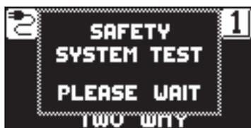
When switching back from the NIGHT LOCK or MANUAL program to the automatic program, the automation carries out the safety system test.
