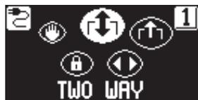
Pressing briefly the button **VSETA**, select the automatic door operating mode. Whenever the button is pressed, you switch from a work program to the next. The display sequentially shows the available work programs.
