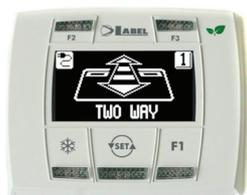
Pressing with a pulse the button
