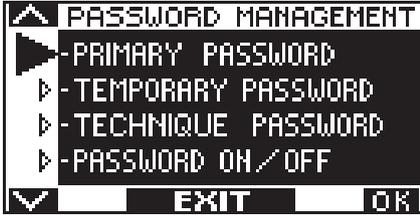
This section displays the two passwords available to the final user, the primary password and the service password.
