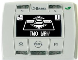
Pressing briefly the button
